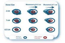
Respiratory movements cause the renal stone to shift out of the focal zone making precise stone positioning frequently intricate. With one of the largest focal zone in the industry (13x60mm), the E3000 large focal area improves stone fragmentation, and drastically reduces all negative effects of the respiration-induced movements.
